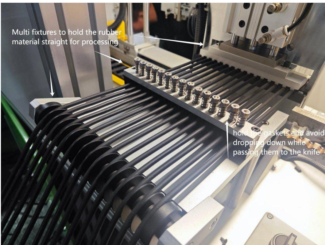
Multi fixtures to hold the rubber material in straight and parrell line for processing .
