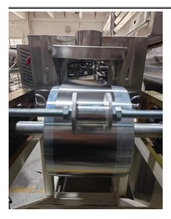
**6, Optional feeder device on top of the extruder ,a**dopting roller type feeding, the feeder speed are matching with
