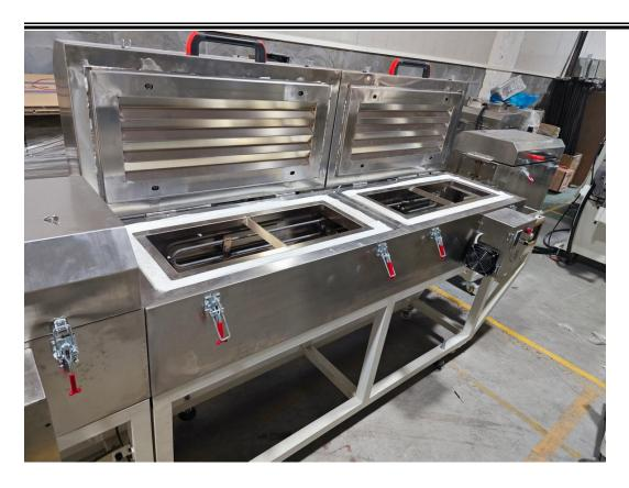
The heating tunnel applies with double-cover on top which is more airtight and does not deform at high temperatures. It is made of stainless steel  $304\,\mathrm{and}$  is cleaner and more nice .
