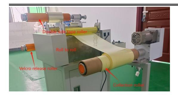
**2,Air blooming winding roller**, the velcro with 3m tape joining and winding machine applies with air blooming winding roller
