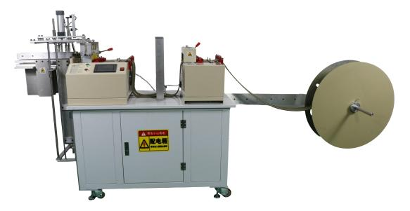
The maximum stacking length is 400mm and can be customised , the stacking height is 230mm and can be customised , two pcs of 90mm width at maximum can be cut and stacked together . the holder boards can hold velcro roll diameter up to 500mm , the velcro ID is 25mm and can be customised based on customer requirements . the machine power is 1000W ,the cutting motor applies servo motor and the feeding machine applies close loop stepping motor
