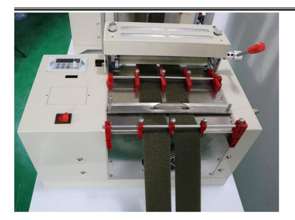
${\bf 4, Holder \ boards}$  , the holder boards is 500mm diameter , it can hold velcro roll up to 500mm diameter and two velcro roll can be
