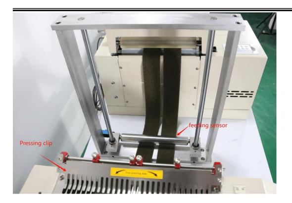
The pressing clip press velcro beneath it , when the velcro material runs out , the pressing clip fall down into the machine and raise alarm to remind
