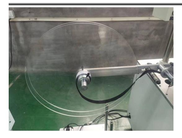
**2,Count meters** this self adhesive velcro cutting coiling roll machine can count how many meters of velcro material had been processed for better recording purpose .
