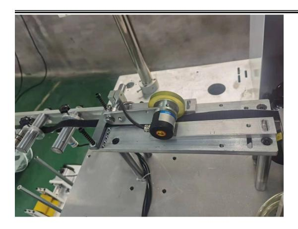
**3, Clipping hands & taping ends** ,the clipping hands will draw the velcro to the cutting knife and cut off , winding device will wind velcro into rolls and tape up the ends to form a fixed velcro rolls .
