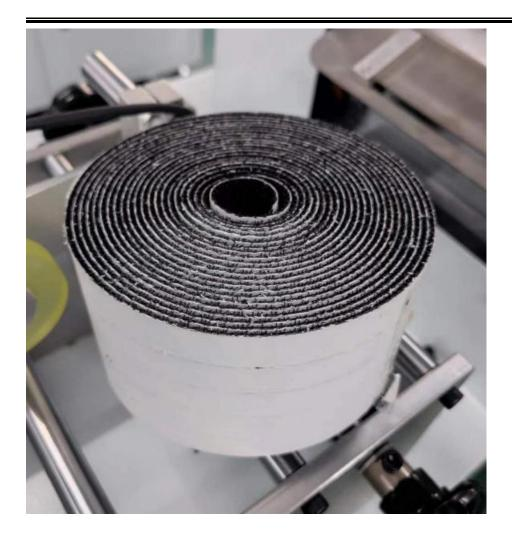
The Maximum velcro  $\,$  material diameter before processing is 800mm and maximum velcro material diameter after coiling is 130mm , the maximum processing material width is 120mm ,the machine can slit big width velcro into small width velcro before coling into rolls , the minimum slitting width is 8mm .
