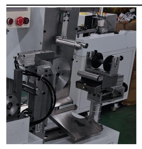
**4, Slitting and cutting velcro to length** , the velcro automatic cutting and winding machine can slit velcro into
