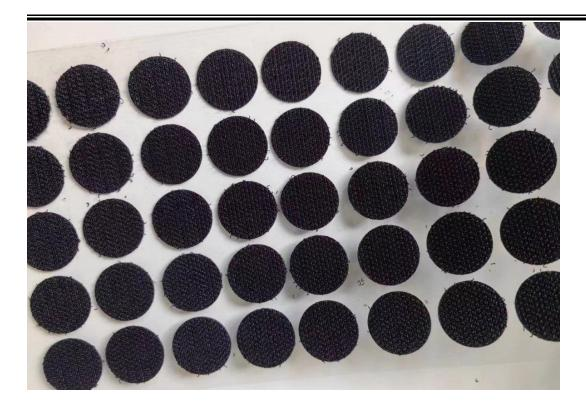
The maximum velcro material cutting width is 150mm and mold length is 120mm, customer can decide their velcro sizes, velcro coins diameters or other irregular shapes with CAD drawings if possible, we will customise the knife molds for customer, the knife molds are very cheap cost which allow customers can work for many different sizes velcro shapes.
